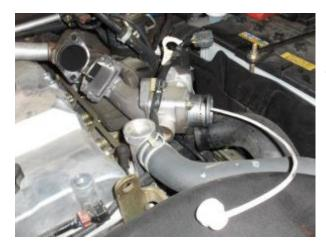
C2. If the valve is at remote distance to the injection point of the product, use an extension tube (available in option) to get closer to the valve, then act the same way as in A.
